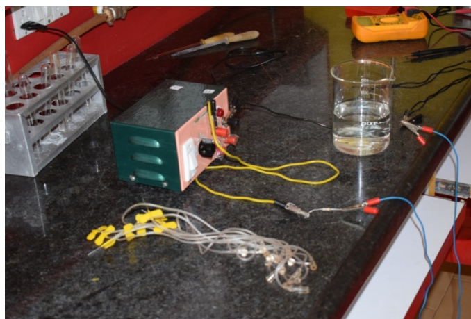
Figure 4: Electrochemistry setup for making electrodes
